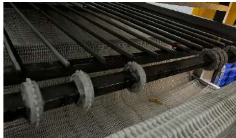
Gambar 4. Perbaikan as conveyor
