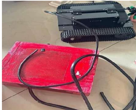
Figure 5. 32V of LiFePo4 batteries with PCM installed
