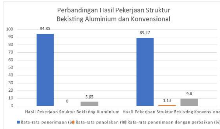
Figure 2. Graphical Comparison of Aluminum and Conventional Formwork Structural Work Results
