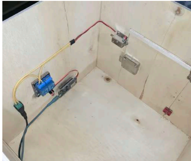
Figure 13. Door Lock Solenoid Test Results Close the lock
