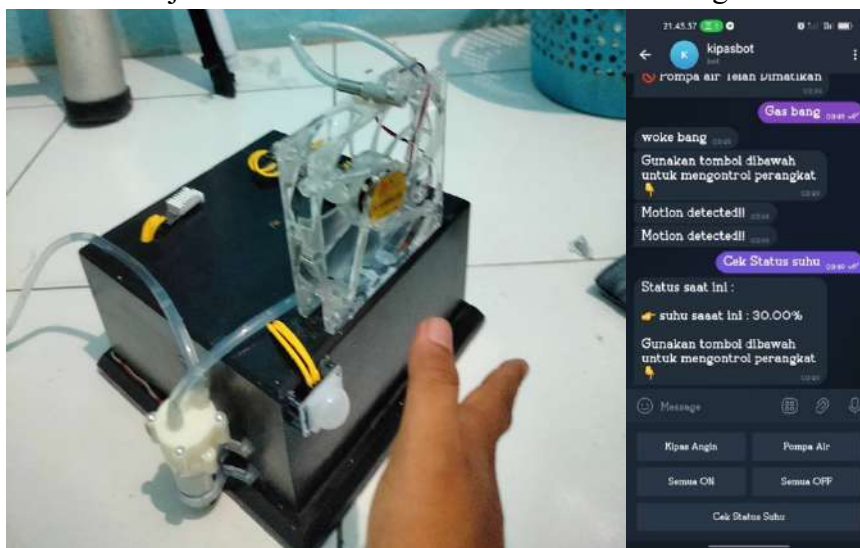
Figure 12. Test results for movement detection sensors
